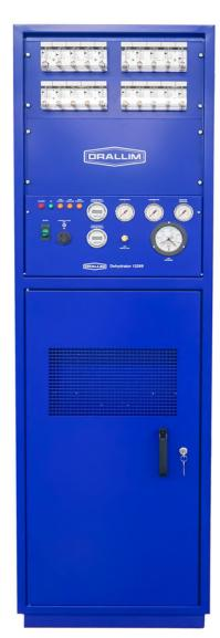
This very high performance unit stands over 2.2m high, and is home to two 3/4HP compressors. Using timers and pressure switches, the compressors are controlled to run alternately when the demand for air is within the capability of one.
