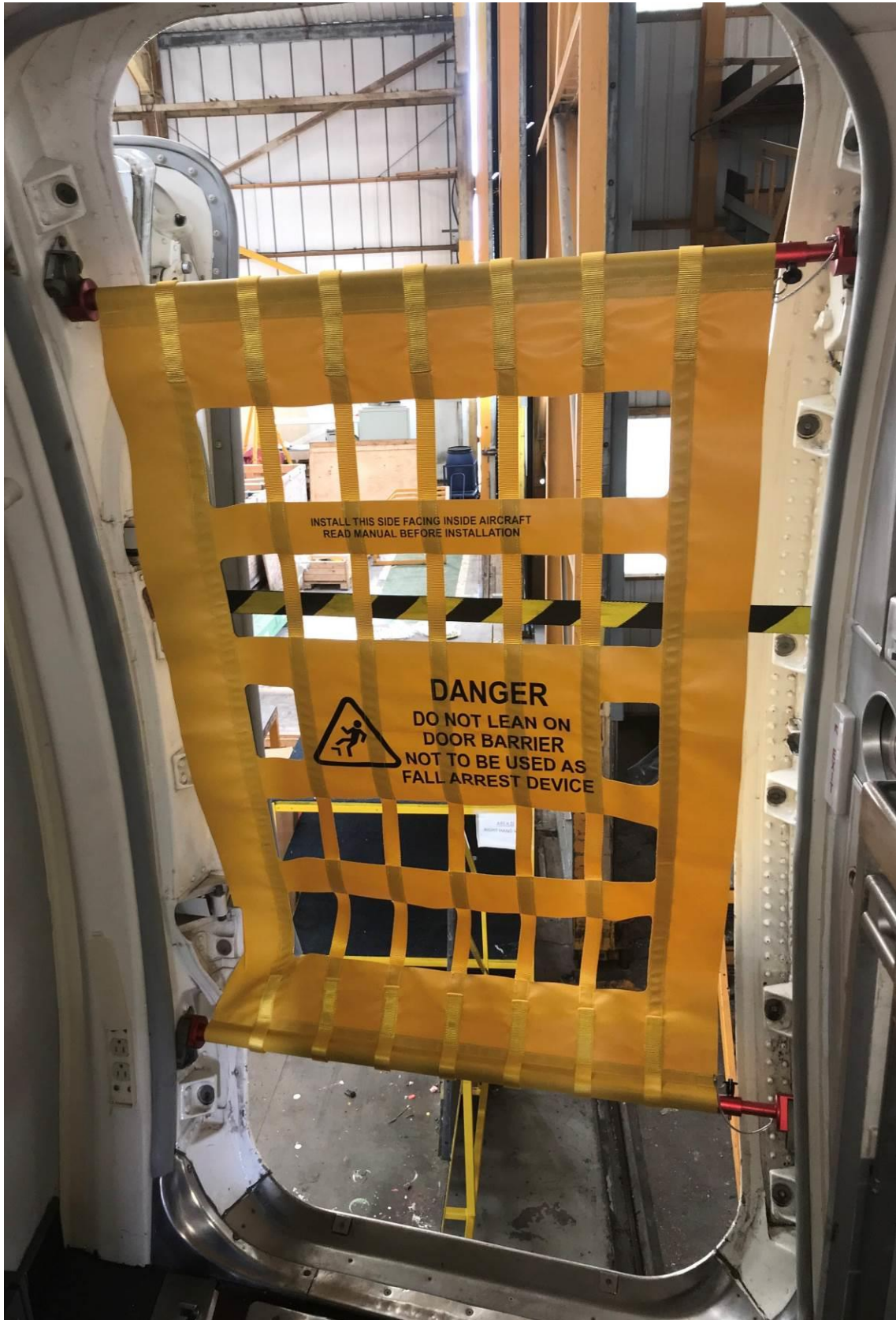
Figure 20 – Door Barrier Part no. 512CA29 installed to Aft Service Door
