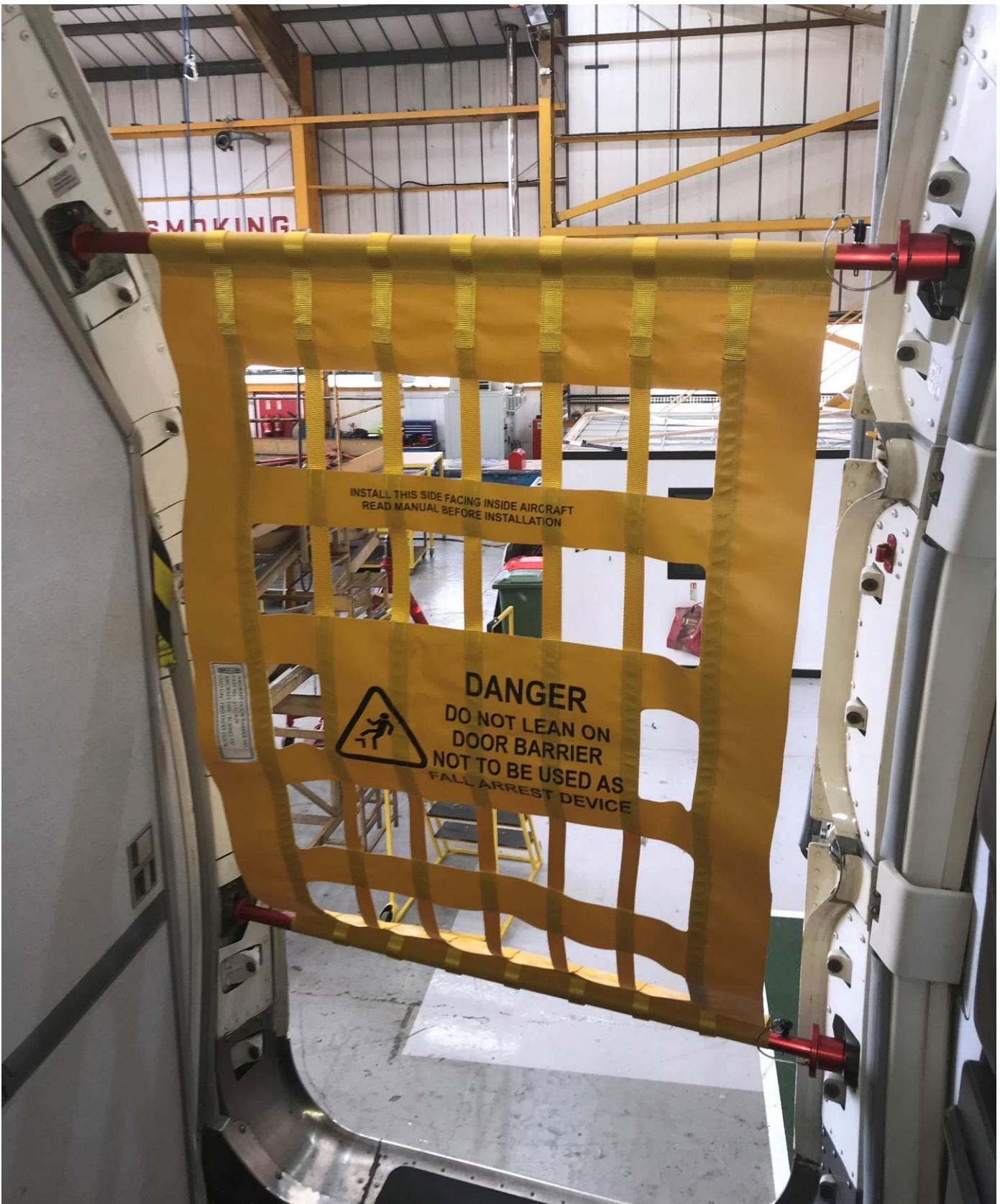
Figure 12 – Installed Forward Entry Door Barrier Part no. 511CA29
