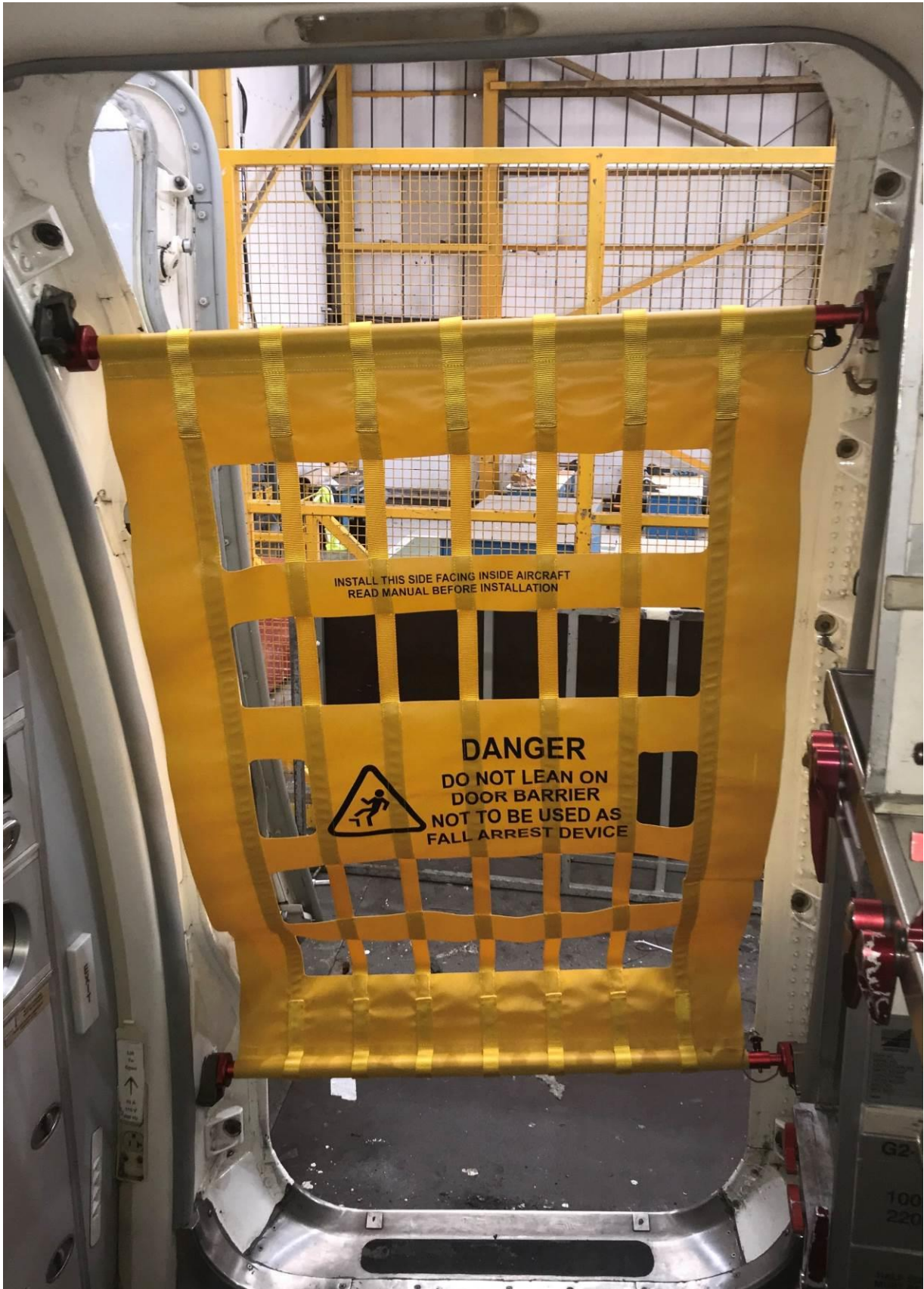
Figure 18 – Door Barrier Part no. 512CA29 installed to Forward Service Door
