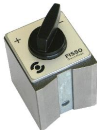
Magnetic base (M8 screw holder; Holding force: 800 N; Base size: 63 mm x 50 mm x 55 mm) (art.# UTM-MAG-0800)
