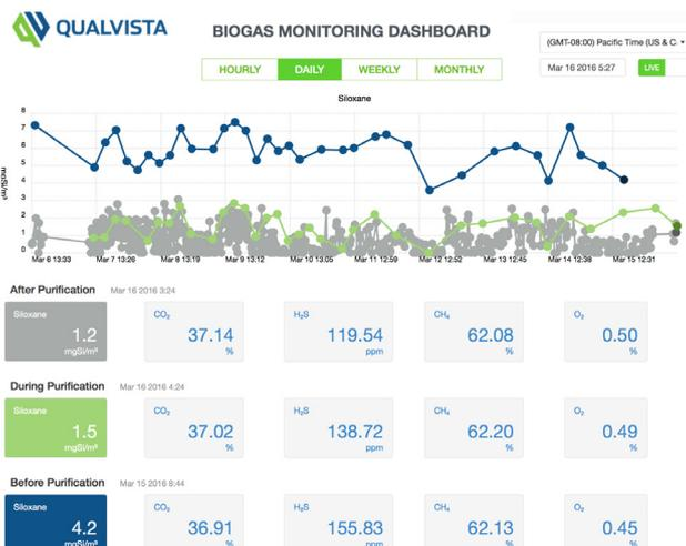
**The Qualvista online reporting tool** gives the user a comprehensive, customizable view of the biogas measurement information, such as siloxane purification efficiency and current or cumulative amount of siloxane entering gas engines or turbines.
