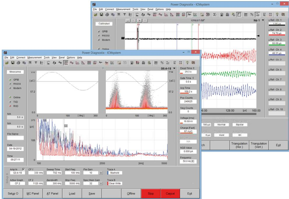
The ICMsystem's PC software includes convenient options for in-depth analysis and printing of stored PD patterns.
