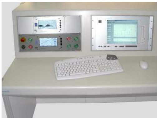
HVcontrol embedded in a control desk
