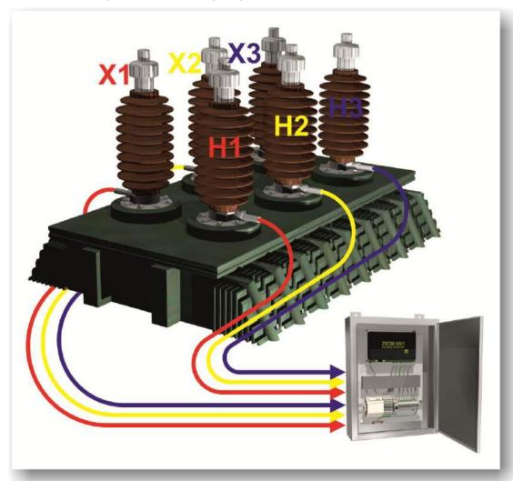
Bushing failures are considered as one of the major causes for transformer outages. Historically bushings were tested off-line to measure the capacitance and the dissipation / power factor.
